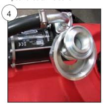
Insert coupling into inlet of pump ensuring the coupling is fed through the captured nut first.
