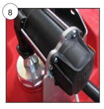
Install pump and attachments into tank inlet hole using captured nut to secure to tank. Pump head will then be positioned on the support bracket. To secure use m5 screws
